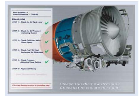
Pratt & Whitney used Right Hemisphere's Deep Creator and Deep Server to develop a real-time, interactive diagnostic system for troubleshooting aircraft engines.
